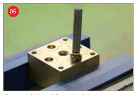
Countersink the  $\emptyset$  8.5 mm boreholes to  $\emptyset$  9 mm x 90°.
