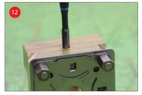
If EWIS<sup>TM</sup> Chips are used for automatic holder identification, then the thread must be fitted to the reference side (chip ER-094168).
