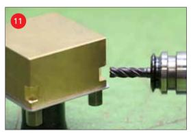
If the retrofitted ITS 50 Holders C are loaded by means of a Robot, then the gripper slot must now be reworked.
