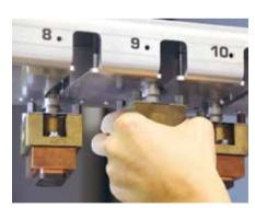
The pass-through, the new and ingenious solution to magazine loading with electrode holders. The holders are loaded and replaced from the operator's side of the magazine.
