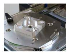
Turntable with 4x90° indexing and pallet lock.
