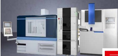
EROWA Robot Compact 80 between an EDM machine and a milling center.
