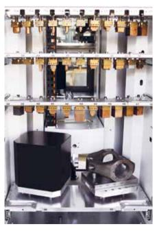
The rack magazines are configured as demanded. Mixed operation of different pallets is possible.
