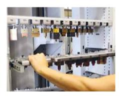
Easy loading and unloading by pull-out magazine drawers. The pull-out is triggered by the integrated handle positions.
