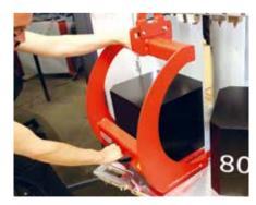
The pull-out magazine levels are also convenient for loading the magazine with an EROWA lift or an overhead crane directly to the magazine position.
