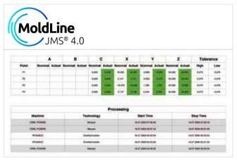
Log | And if anyone wants to know exactly what the target/actual comparison results are, the specific workpiece log has all the information. It is directly accessible from JMS® 4.0 MoldLine.
