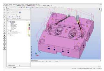
**CAM!** CAD data is imported via the interface to the CAM. JMS® MoldLine receives the programs and assigns them to the workpieces.
