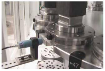
**Identification** I Staged pallets with workpieces are uniquely marked with a chip. At every station in the production process, each pallet is precisely identified by the EROWA EWIS™ system.
