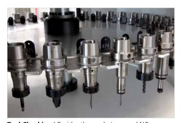
Tool Checking I Besides the workpieces and NC programs, you need the right tools as well. Whether this is the case, and what their remaining lives are, is read from the memory of the machine.
