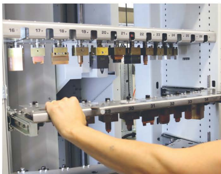
Easy loading and unloading by pull-out magazine drawers. The pull-out is triggered by the integrated handle positions.
