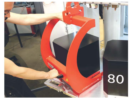
The pull-out magazine levels are also convenient for loading the magazine with an EROWA lift or an overhead crane directly to the magazine position.
