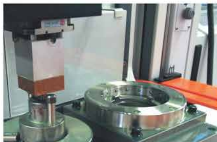
EDM Shapes on the surface of the punches and dies are EDMed.
