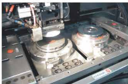
Wire-EDM Continuous contours in dies and punches are machined on the WEDM machine.
