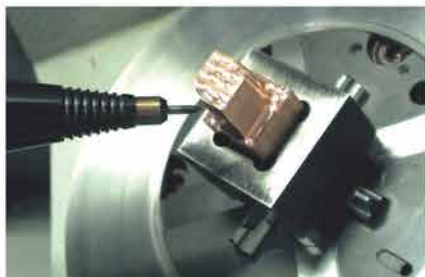
Milling Electrodes for EDMing the forms are produced on ITS system holders.
