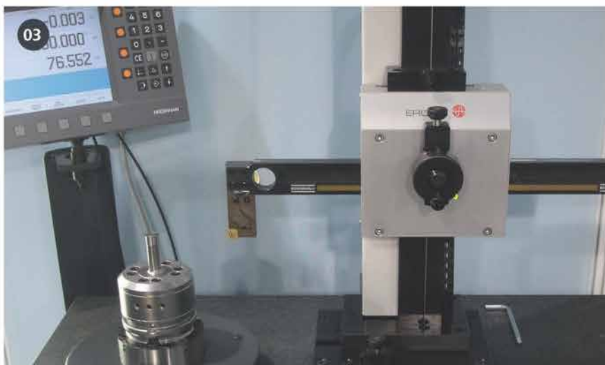
The pallet is clamped pneumatically on the alignment device – Repeatability < 0.002 mm.
