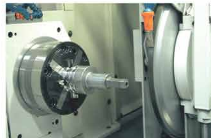
Grinding Punches can also be produced on circular grinding machines.
