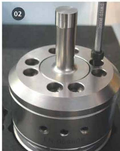
The punch can then be mounted and clamped in the adaptation pallet.
