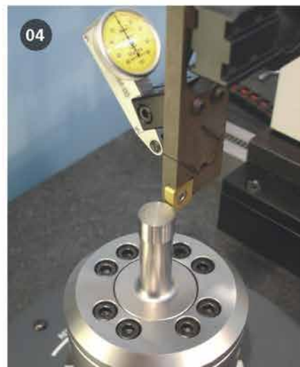
The punch is aligned with absolute precision to the system datum point.
