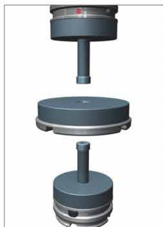
Release and remove die, bottom and top punches pneumatically.
