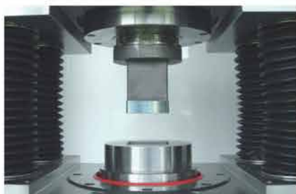
Powder presses Top and bottom punches and the die are inserted into the powder press. The reference positions are given by the precisely aligned chucks.
