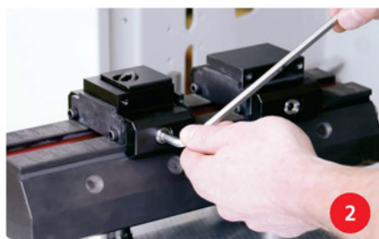
Position and fasten the clamping element based on the size of the workpiece.
