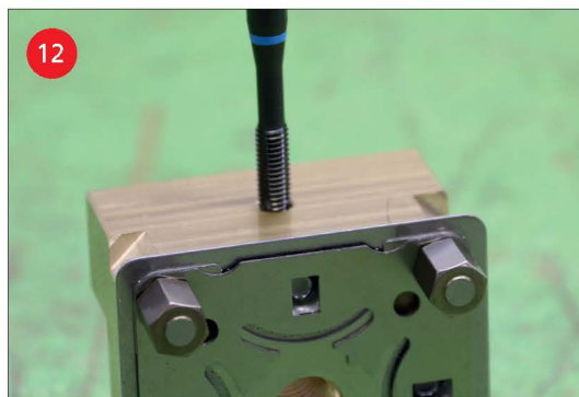
If EWIS™ Chips are used for automatic holder identification, then the thread must be fitted to the reference side (chip ER-094168).
